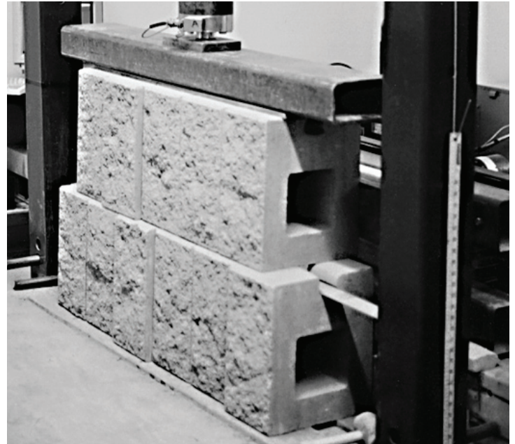
Connection test apparatus with Landmark® modular units.
